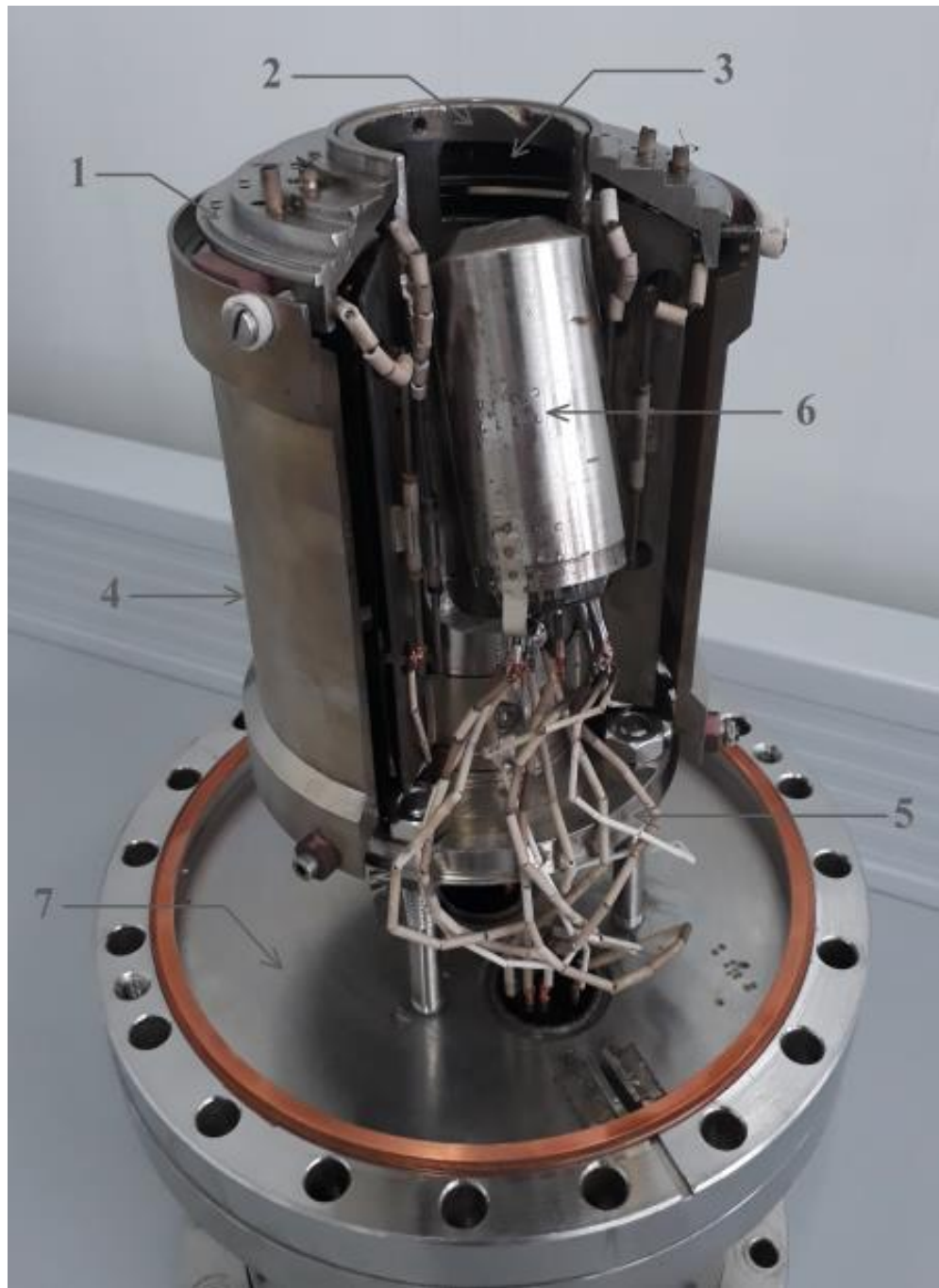
1- face electrode, 2- inner cylindrical electrode, 3- inlet window, 4- external cylindrical electrode, 5- back electrode, 6- electron gun, 7- high vacuum flange
