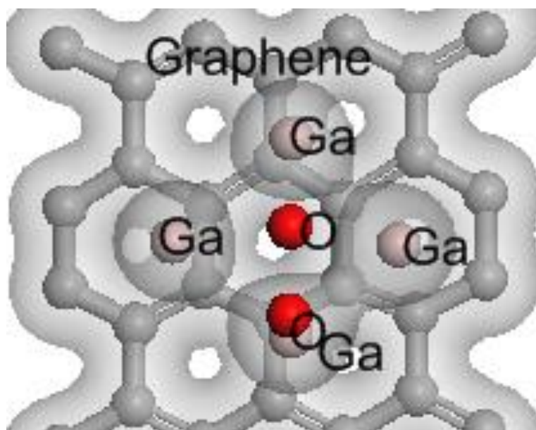
Figure 28 – Possible stable structure of a graphene protective coating element with a gallium cluster with an adsorbed oxygen molecule
